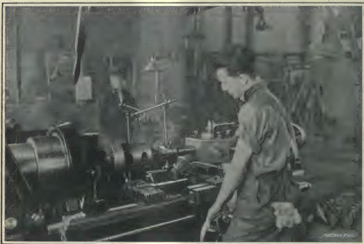
Fig. 16. Third Operation on Nose of Shrapnel Shell—Turning, Facing, and Threading
